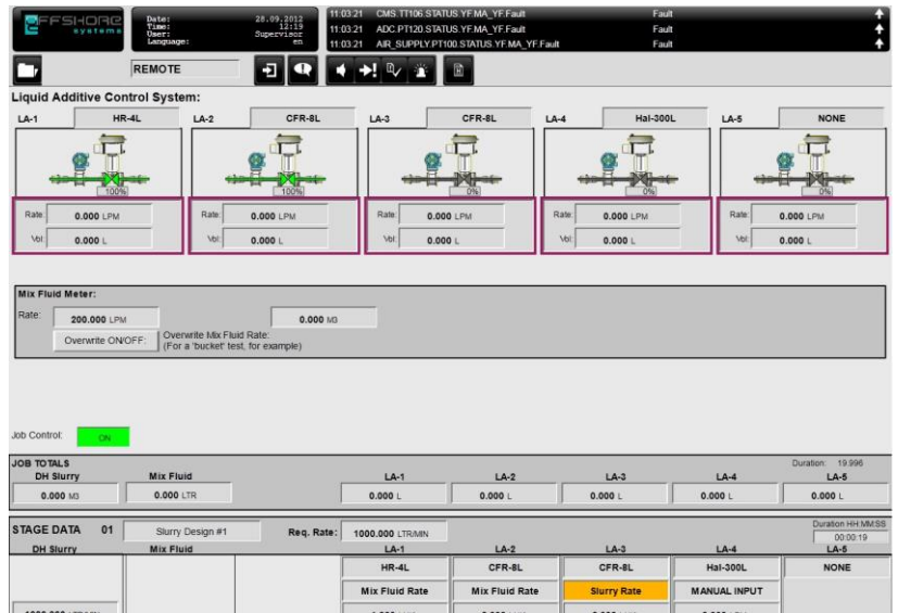
Atvise HMI picture showing set up of the Smart Flow unit.
